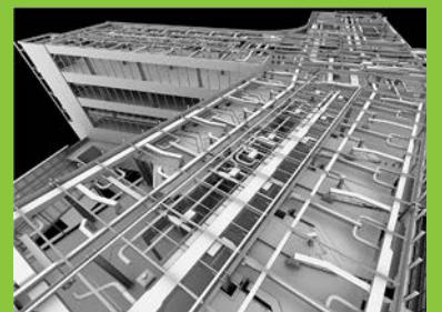
Building Information Model (BIM) of the mechanical/electrical/plumbing (MEP) corridor racks
