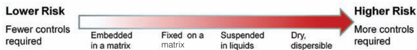
FIGURE 4.5 U.S. Department of Energy graded exposure risk for nanomaterials. This figure assumes that no disruptive force (e.g., sonication, grinding, burning) is applied to the matrix. SOURCE: Adapted from Karn (2008).
