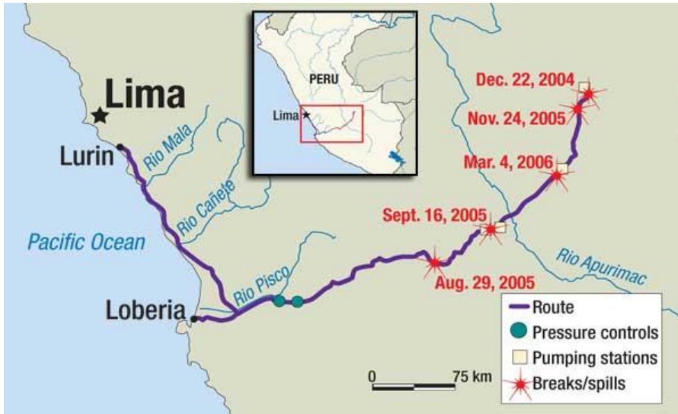
Figure 4. Diagram of pipeline spills within the first 14 months of operations. Source: Schexnayder, C.J. Engineering News-Records (March 16, 2006). “Despite Explosion, Peru Pushes Forward with $2B LNG Project.” Accessed on April 1, 2013. http://enr.construction.com/news/intl/archives/060316.asp .
